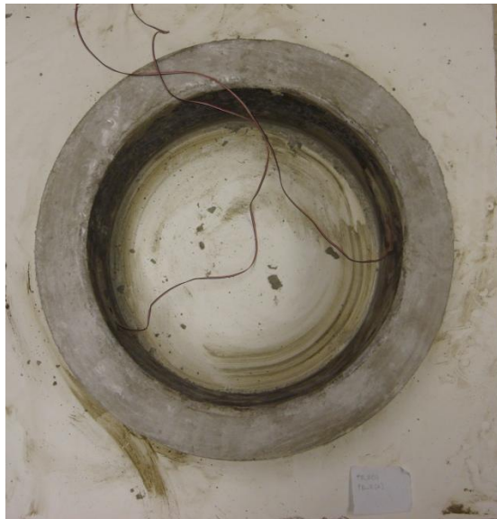
Figure 15 Configuration of restrained concrete ring samples.
