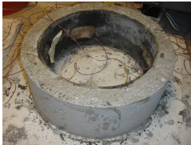
Figure 21 Configuration of restrained concrete ring samples.
