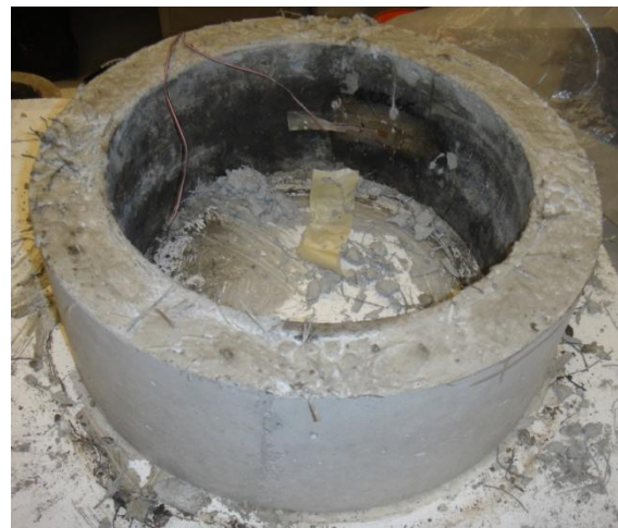
Figure 19 Configuration of restrained concrete ring samples.
