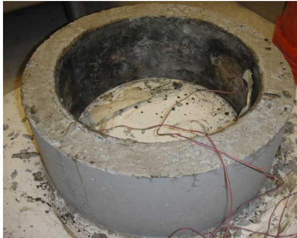
Figure 16 Configuration of restrained concrete ring samples.
