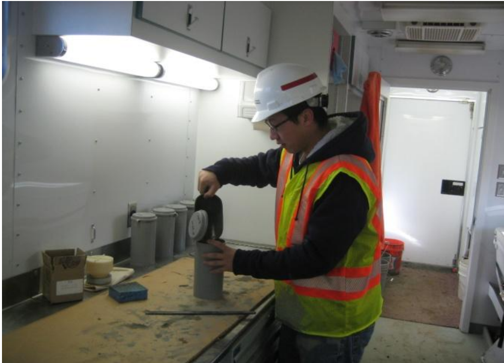
Figure 8 Preparing concrete cylinder samples.
